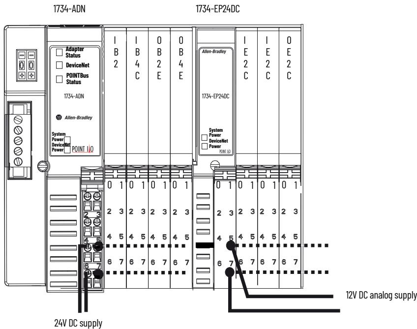
**Specifications****POINT I/O 24V DC Expansion Power Supply – 1734-EP24DC, 1734-EP24DCK**
